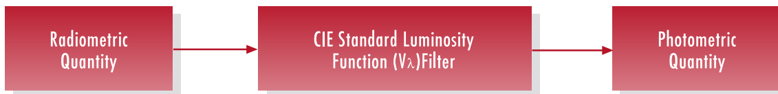
Fig. 2.3b - Relationship between radiometric units and photometric units
