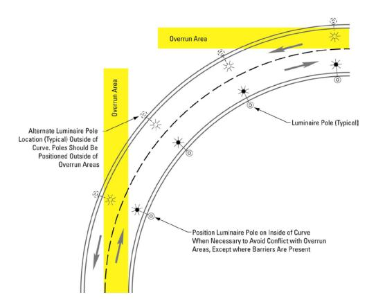
Figure 38 – Pole Spacing on Curves
