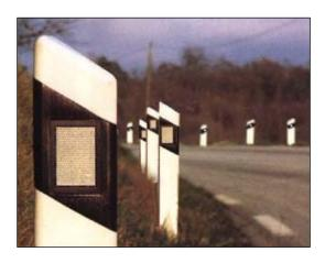
Figure 41 – Post-Mounted Delineators (PMDs)
