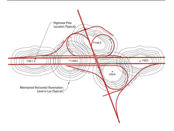
Figure 33 - Highmast Pole Spacing
