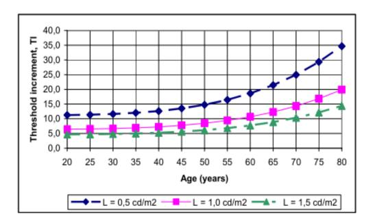
Figure 26 - Impact of Glare and Light Level on the Visibility of Aging Drivers
