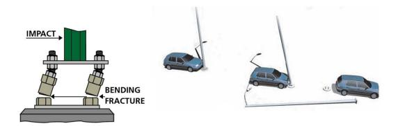
Figure 39 – Pole with Breakaway Device
