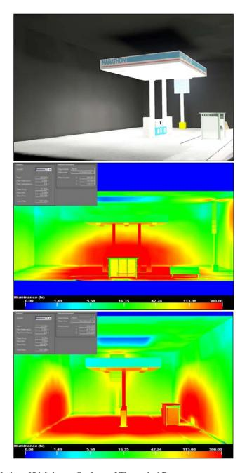
Figure 35 - Example Calculation of Lighting on Surfaces of Theoretical Box
