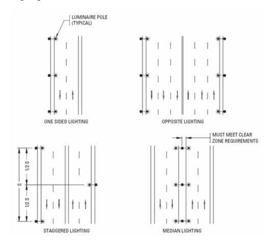
Figure 31 – Typical Pole Spacing
