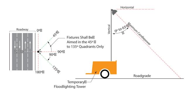
Figure 44 – Work Zone Floodlight Aiming
