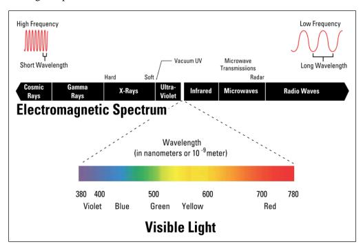
Figure 4 - Electromagnetic Spectrum and Visible Spectrum
