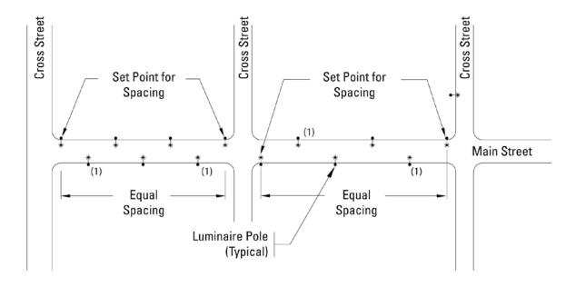
Figure 32 – Pole Spacing
