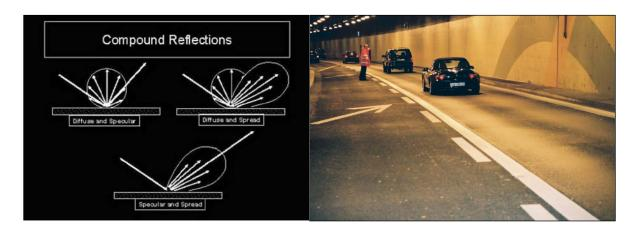
**Figure 16 - Pavement Reflective Differences**
