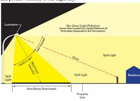
Figure 18 - Spill Lighting, Glare and Skyglow
